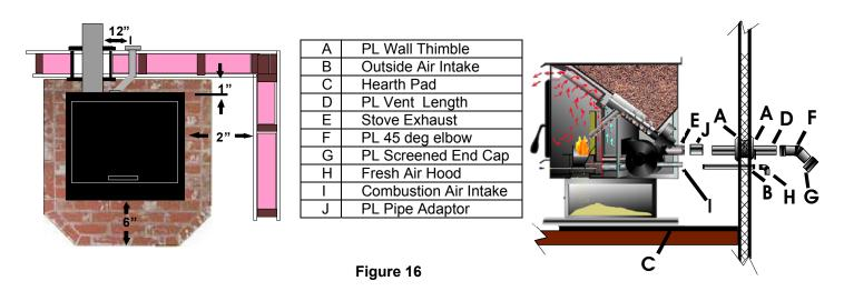
NOTE: Some horizontal, through the wall installations may require a Clean-Out Tee and a minimum 3' vertical rise of pipe outside the building to help draft the stove. This is required if a proper burn cannot be maintained, after the stove has been tested and the airflow set. This is due to backpressure in the exhaust, caused by the airflow around the house.
